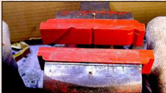
Fig. 4. These plastic jaw inserts have imbedded magnets to help retain them on the vise. Note the grooves at vertical, horizontal and 45° to prevent slippage of small diameter work pieces.
