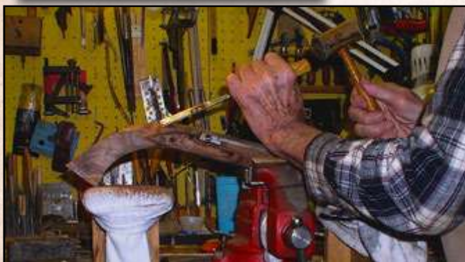
Fig. 14. Whether right side up or upside down, the adjustable support will keep the fore end of the pistol from twisting in the vise.
