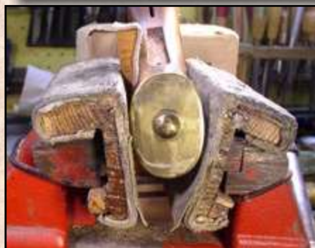
Fig. 13. The vise jaw inserts cock to form a V under pressure to keep the butt from slipping down. Note that one concave insert takes up slack at the narrowing of the butt.
