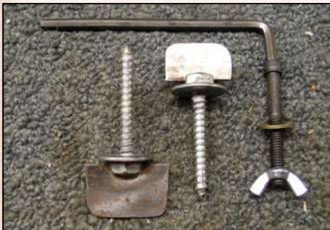
Fig. 8. Washers and thumb tabs are silver soldered to 5/16 x 2" lag bolts (left) and screwed through 7/32" holes.
