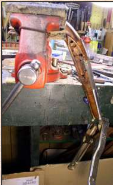
Below: Fig. 12. For engraving the rounded corners of the cap, I secured the butt in the vise with the aid of two concave, leather-covered inserts I use for horn work.
