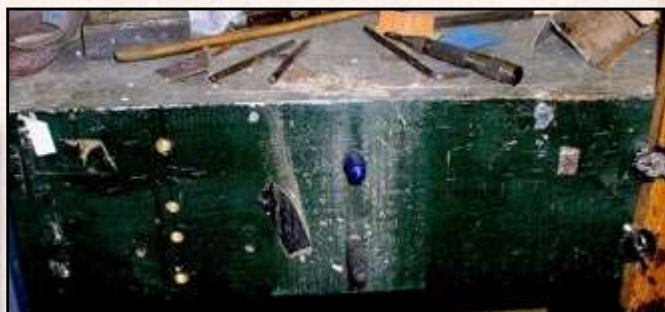
Fig. 5. The fascia board of the workbench is used for attachments of various supports. The cap bolts that protrude are sharp and should be covered with rubber tubing when not in use to prevent injury.
