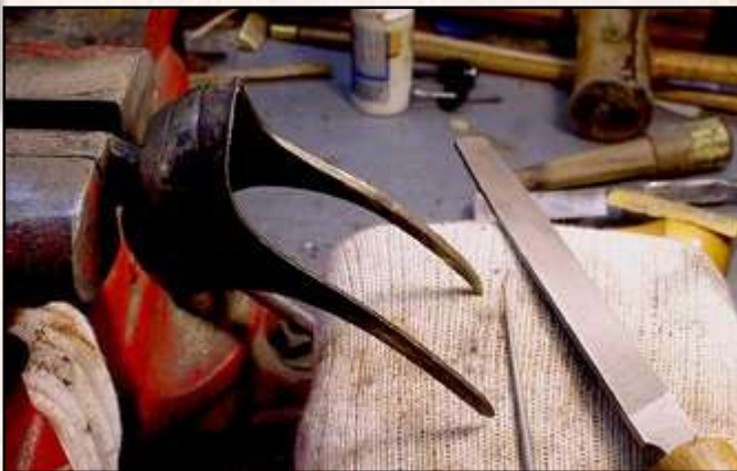
Fig. 16. Those long, tangs won't take much pressure, but the big hunk of metal at the butt will stand as much pressure as a vise can exert.
