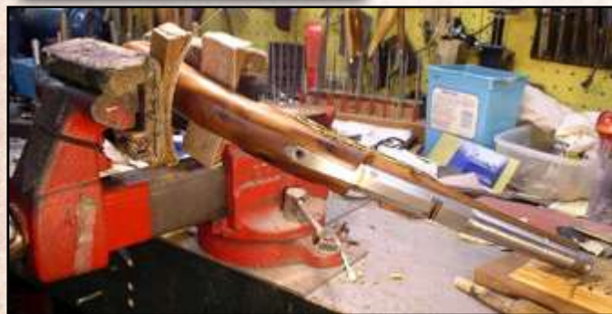
Fig. 13. The vise jaw inserts cock to form a V under pressure to keep the butt from slipping down. Note that one concave insert takes up slack at the narrowing of the butt.
