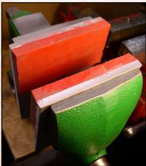
Fig. 17. This Multi-Vise is heavy-duty construction and made in the USA. Unfortunately, it requires the construction of a support that holds its base in a vertical position to achieve the to-and-from rotation that positions the pistol at the most advantageous work angle.
