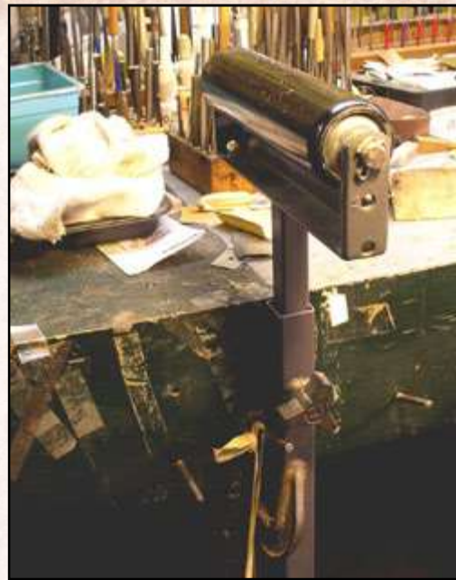
Fig. 9. This roller support by Keith Lisle is easily moveable and versatile for support of pistols or rifles.
