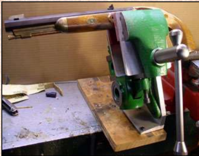
Fig. 17. This Multi-Vise is heavy-duty construction and made in the USA. Unfortunately, it requires the construction of a support that holds its base in a vertical position to achieve the to-and-from rotation that positions the pistol at the most advantageous work angle.
