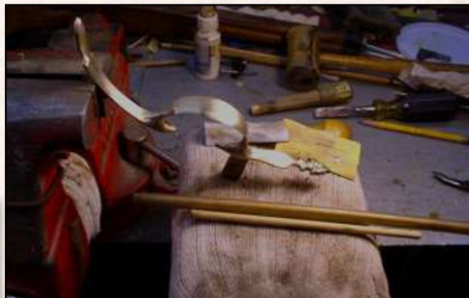
Fig. 15. Pinning tabs are the only parallel-sided structure on trigger guards that provide firm purchase points.
