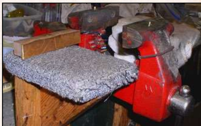
Fig. 6. These homemade supports were made of one-inch oak. They are adjustable for height to support the work piece on both sides of the vise. Note the backstop on the padded top of the support. It is faced with buffalo leather and has a dowel that can be inserted into the support and pivot to conform to the work piece.
