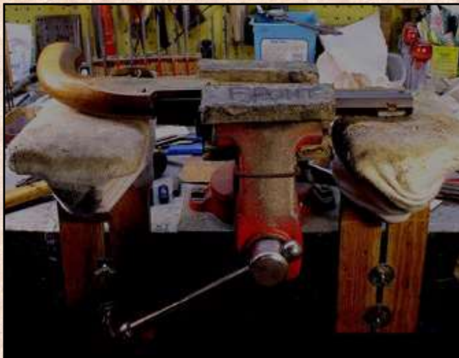
Fig. 1. This clamping arrangement of bench vise and home-made rests has been used for pistol work for many years.
