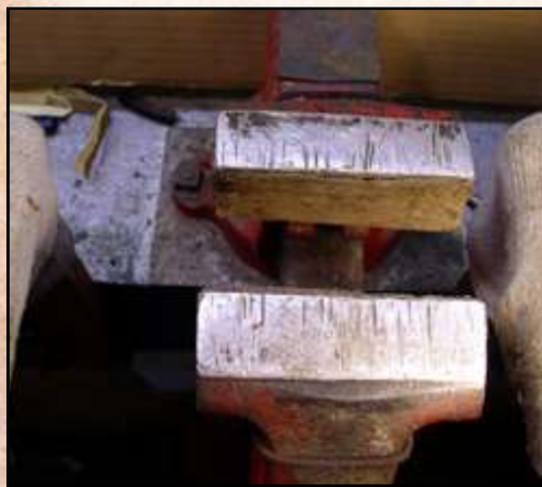
Fig. 3. These jaw inserts were made from 1-1/4" x 1-3/4" aluminum angle. They are lined with 0.015-inch thick "shirt board" to prevent aluminum smudges on gun parts and to protect the clamped work piece
