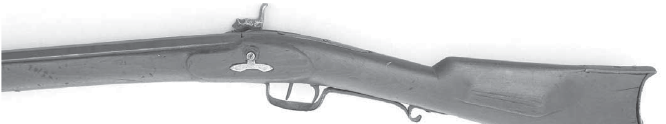
Figure 9b - The reverse of Shell's rifle has a small, inverted "T" lock bolt washer that is reminiscent of Tennessee rifles. There are a Kentucky-style two-screw tang, shallow side facings, and an almost crude cheekpiece. No molding lines are present. Shell supposedly won many shooting matches with this rifle, and in later years as his mind weakened, he used the rifle to chase away "flying spirits" or "haints" from his house. Courtesy M. Clark.
